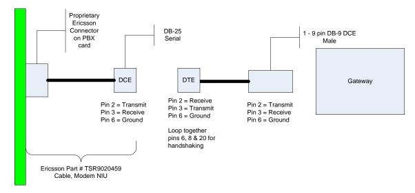
The industry rule of thumb for RS232 serial communications is to keep the length of the cable no longer than 50 feet. Lengths longer than the recommended standard may need additional equipment to ensure correct transmission levels are maintained.
