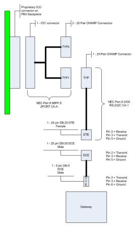
The industry rule-of-thumb for RS232 serial communications is to keep the length of the cable no longer than 50 feet. Lengths longer than the recommended standard may need additional equipment to ensure correct transmission levels are maintained.
