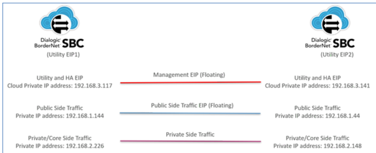
Figure 3: Floating IP Addresses for HA (Secondary)
