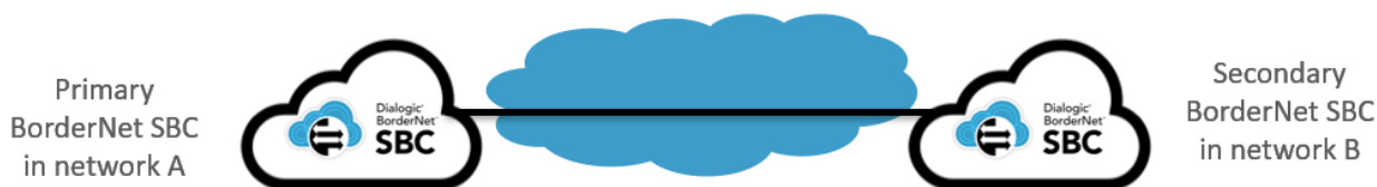
Figure 3-9: BorderNet in Geo-Redundancy Mode
